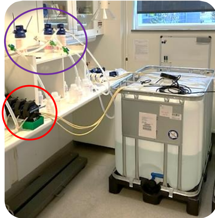
Figure 3 Experimental setup. The container with water containing DPC is shown on the right, and the three filters (triplicates) (purple circle) and the pump (red circle) are displayed on the left. For close-up of the experiment, see “flowchart”.
